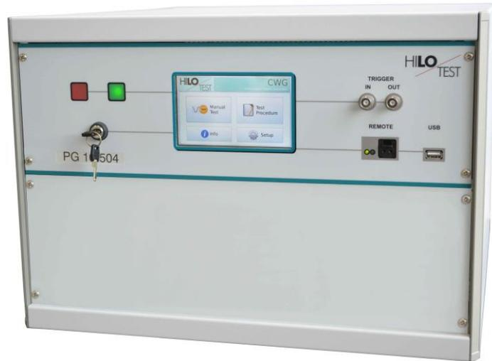
The Combination Wave Generator PG 10-504 is a combined impulse-current-/impulse-voltage generator which, for high-impedance loads,  $R_L > 100\Omega$ , delivers a standard impulse voltage with waveform 1.2/50 $\mu$ s and, for short-circuited output, a standard impulse current with waveform 8/20 $\mu$ s.
