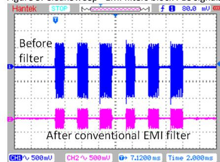
Figure 6. Conventional multistage EMI filters cannot block PLC signals
