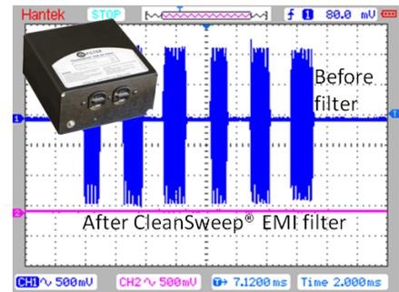
Figure 5. CleanSweep® EMI filters block PLC signals
