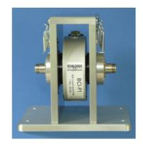
The calibration jig is used for insertion loss measurement of the Bulk Current Injection Probes and meets ISO 11452-4 and IEC 61000-4-6 standards.
