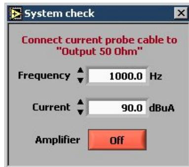
⦿ An output sine wave can be generated at a certain **Frequency**. The setting **Current** defines the applied current when the **Amplifier** is switched **On**. **Off** switches the signal off again. The generated signal may be measured by choosing **Measurement/Acquire once** for one measurement or **Measurement/Acquire on** for continuous measurement.
