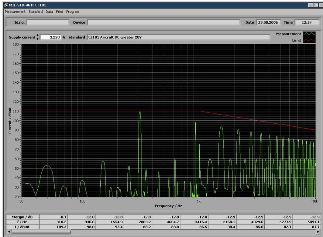
Measurement of DC driven equipment with 3.22 A load current
