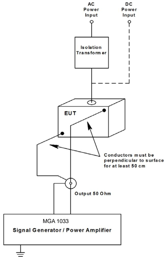
**FIGURE CS109-2. Test configuration.**
