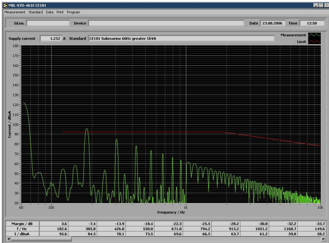
Measurement of AC driven equipment with relaxed limit curve
