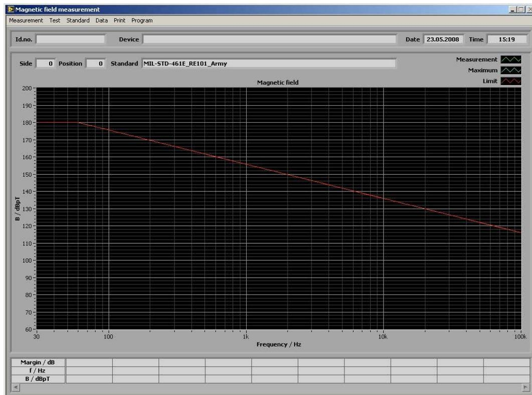
*Magnetic field measurement window with limit curve corresponding to the standard file loaded*
