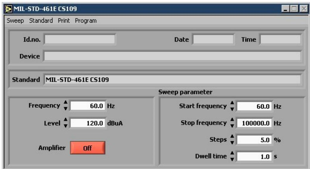
Window for testing according to MIL-STD-461E/F CS109
