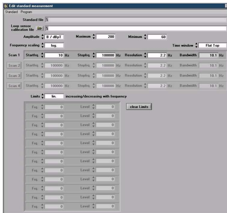
*Edit standard measurement window for limit curve generation*
