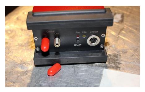
The optical fibers also have red protectors which should be applied when the fibers are not in use.
