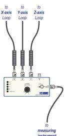
The loops are constructed from high quality RG 223/U coaxial cable, inside flexible 1" PEX pipe. The three (3) loops connect to three (3) current to voltage transducers, the outputs of which connect to three respective inputs on a coaxial switch.
