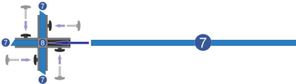
Figure 6 - ALT-930-2M Triple Loop Antenna Assembly – Step #2
