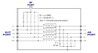
The frequency range of the test is from 150 kHz up to either 80 or 230 MHz. The test level is typically 1, 3 or 10 Vrms with the test signal 80%, AM modulated with a 1 kHz tone. A typical test setup is illustrated below.
