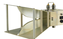
AHA-118 Active Horn Antenna (1-18 GHz)
