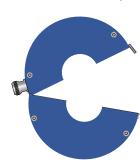
rugged, circular enclosure. The probe enclosure is hinged, allowing the probe to be opened on one side in order to easily place the wire, cable(s) or cable bundle(s) to be tested into the probe window. This makes the CLCE-452 much more convenient to use than other non-split core probes.
