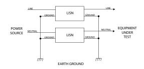
Three Phase connection with two sets of LISNs
