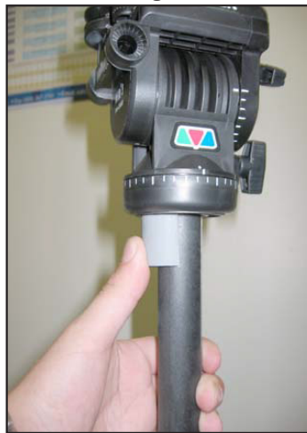
Attach vertical spacer
