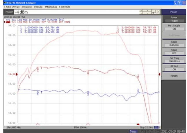
Plot 4 – ALC Flatness @ 52dBm & 45dBm
