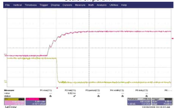
Plot 7 – Switching Time OFF Scale: 0.1μs/Div.
