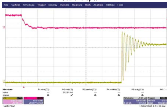
Plot 6 – Switching Time ON Scale: 0.5μs/Div.
