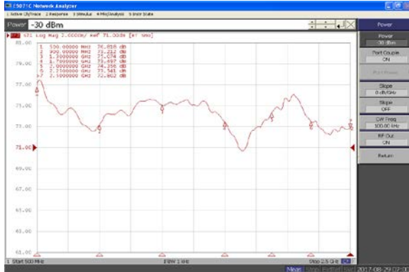
Plot 1 – Small Signal Gain @ P_{IN} = -30\text{dBm} Reference: 71dB, 1dB/div.
