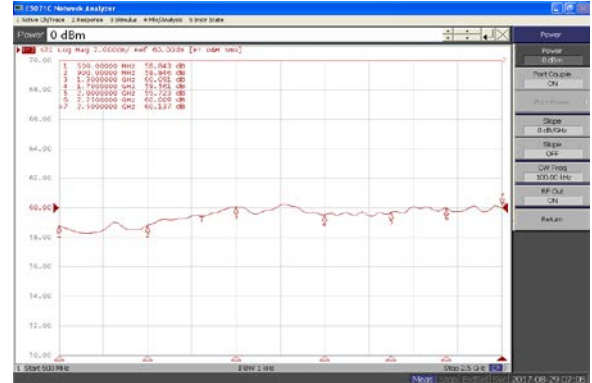
Plot 2 – Levelled ALC Flatness @ 1000W, P_{IN} = 0\text{dBm} Reference: 60dB, 2dB/div/
