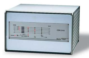
The test set-up is suitable for immunity testing of electronic systems and devices according to IEC 61000-4-4, IEC 61000-4-5 and IEEE 587.
