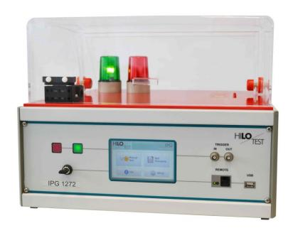
$\,$ HV - Impulse generators IPG 1272 create standard impulse voltages with waveform 1.2 / 50  $\,$ µs acc. to IEC 60. The generators simulate surges caused by switching of inductive loads, power system switching, lightning strokes etc.
