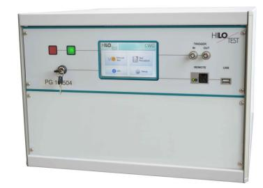
The Combination Wave Generator PG 10-504 is a combined impulse-current-/impulse-voltage generator which, for high-impedance loads, RL >  $100\Omega$ , delivers a standard impulse voltage with waveform 1.2/50µs and, for short-circuited output, a standard impulse current with waveform 8/20µs.
