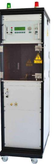
The High Current Pulse Generator type PG 10-7k generates lightning surge currents with the waveform 10 /  $350\mu s$  according to IEC, VDE etc.
