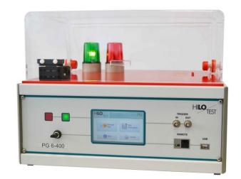
The high current pulse generators PG 6-400 / PG 6-200 are designed for surge testing of electrical components, over-voltage protectors and electronic circuits acc. to IEC, VDE etc. They generate standard impulse currents with waveform  $8/20~\mu s$ . Short circuit output current amplitude is selectable from 0.2 up to 10 kA by adjustment of the charging voltage of the internal energy storage capacitor.
