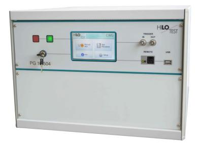
The high-voltage impulse generator PG 6-364 generates standard impulse voltages with waveforms  $1.2/50~\mu s$  and  $10/700~\mu s$ . Output voltage is adjustable between 0.2~kV and 6~kV. The polarity of the output voltage is selectable. Positive, negative or alternating polarity of the output voltage can be preselected.
