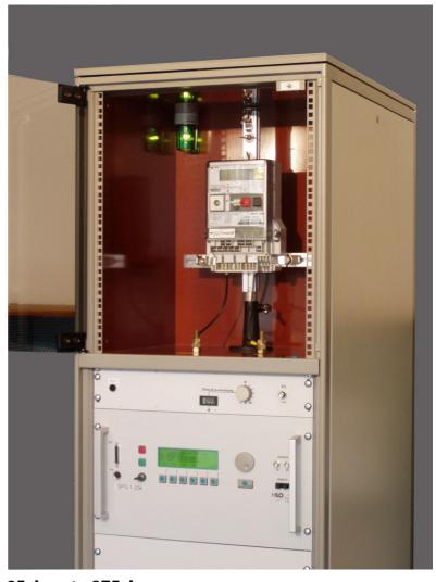
The pulse shaping network comprises an impulse current measuring resistor for the surveillance of the impulse amplitude. The impulse current output is placed on the top of the generator and it is designed as a high current test adaptor.
