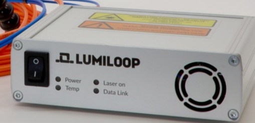
Computer Interface (CI) - with laser unit* and - USB device interface
