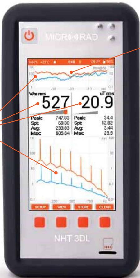
Simultaneous view of the electric and magnetic fields (combined mode menu)
