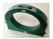
Sensitivity Output resistance Maximum peak current Maximum rms current Droop rate Useable rise time Current time product Low frequency 3dB point High frequency 3dB point High frequency 3dB point I/f figure Output connector Operating temperature Weight 0.001 Volt/Ampere ±1% 50 Ohms 500,000 Amperes 1000 Amperes 0.3 %/millisecond 400 nanoseconds 15 Ampere-second maximum 0.4 Hz (typical) 1 MHz (typical) 70 rms Amperes/Hz BNC 0 to 65 °C 5.5 pounds
