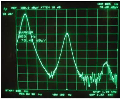
Figure 3a: View of 6.3 Vrms 800 Hz ripple on a 400 Hz 115 Vrms bus, using the PRD-120
