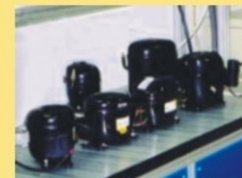
Compressor for Air Conditioner
