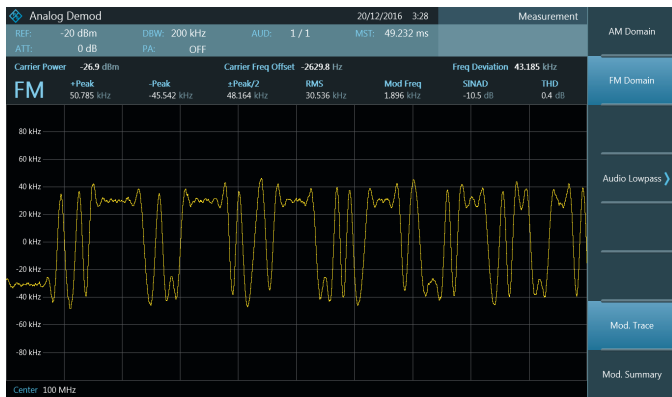
R&S®FPC-K7: FM modulation analysis
