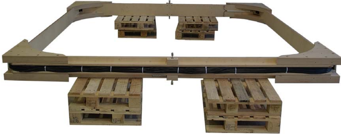
Cable bundle inserted and coil frame ready to lift
