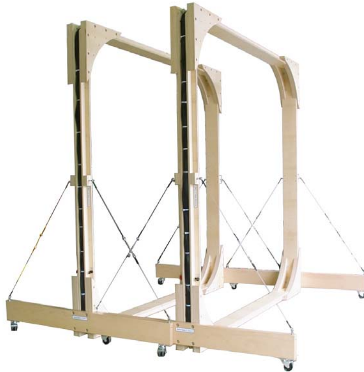
Two coils arranged for the functional test to obtain minimum distance
