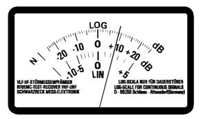
The meter uses the classic 0 dB centre of meter scaling for safe measurement without interpretation.
