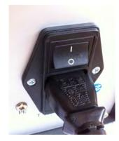
Figure 2.9: Main Switch / Power Socket
