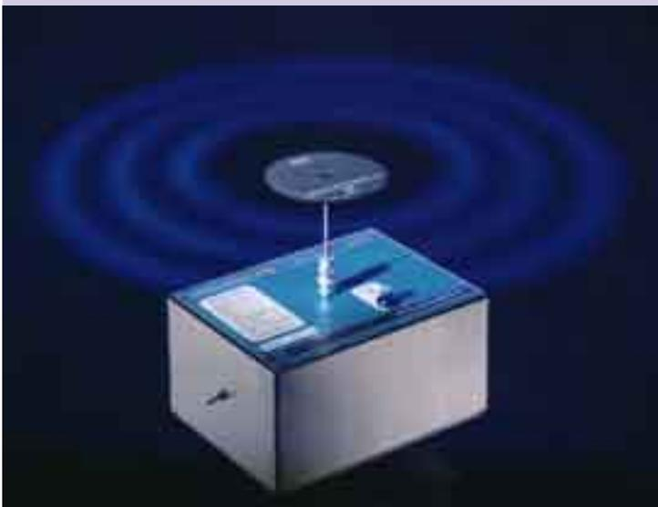
The range comprises two models, the ERS and the EMC10.3G. Each radiate a known RF field strength and are supplied with calibration data measured at 3 metres. Their output is in the form of a closely spaced harmonic series which provides a continuous, narrowband signal covering the whole range. Measurements of these signals are unaffected by receiver RBW of detector type, reducing the possibility of error and ensuring a highly stable result.
