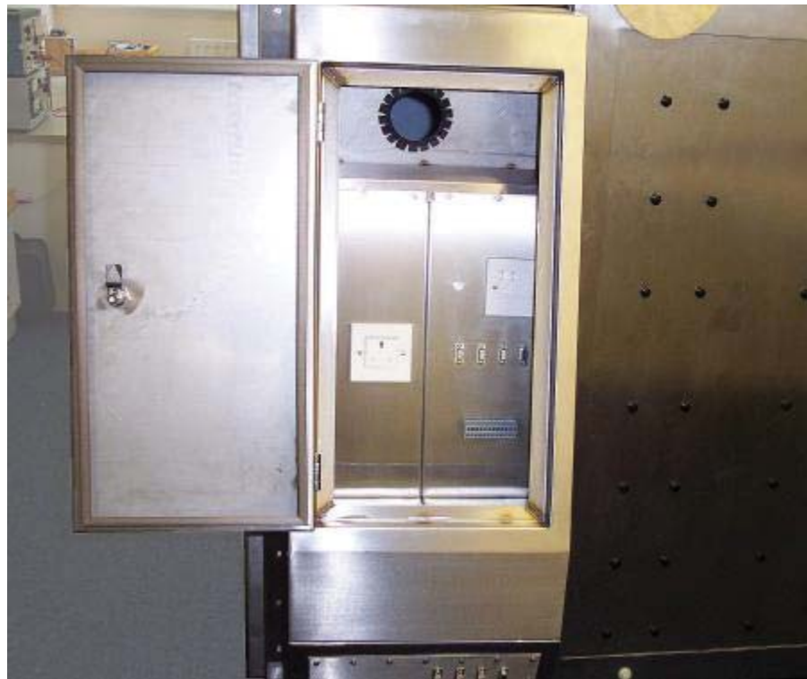
Figure 3 Rear view of cell showing facilities for connections to EUT inside the cell.
