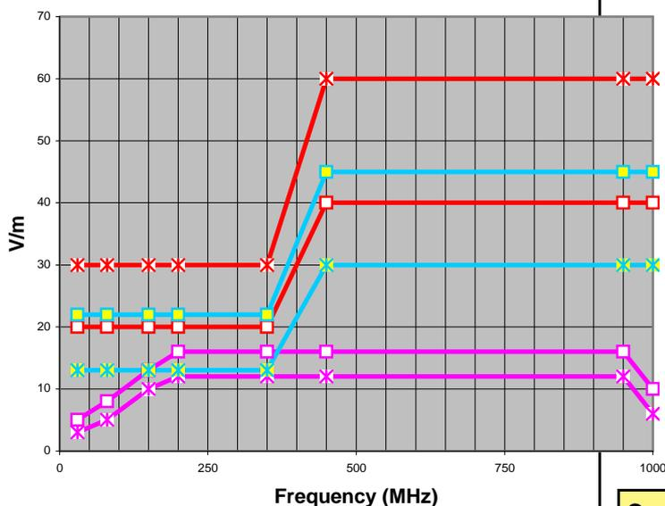
The graph shows actual field strengths achieved in three types of test facility with two of the above amplifiers.
